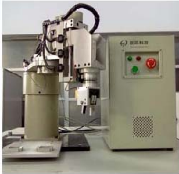
Figure 8. Robot manipulator with three freedoms used in experiment.
